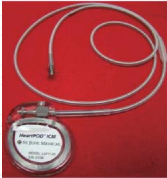
Standalone HeartPOD with communicator module attached to sensor lead
