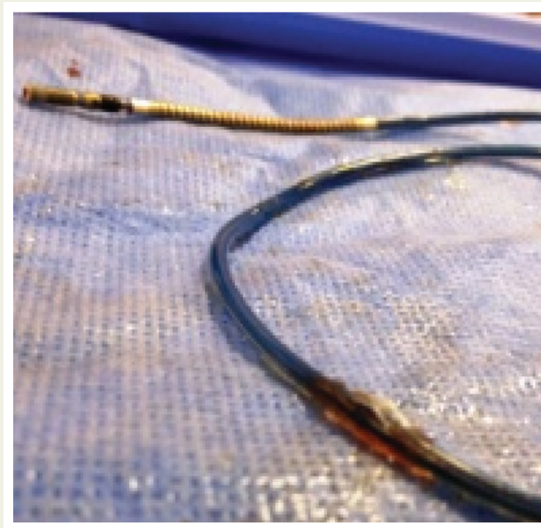
Figure 1 Explanted defibrillator lead showing insulation break.
